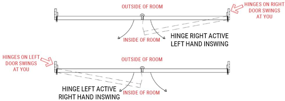
\*INACTIVE DOOR BECOMES OPERABLE ONCE TOP BOLT (INCLUDED) IS UNLOCKED ALLOWING BOTH DOORS TO SWING LEAVING NO OBSTRUCTIONS WITHIN THE FULL OPENING. ACTIVE DOOR MACHINED FOR STANDARD 2 3/4" BACKSET, 2 1/8" DIAMETER HANDLES (NOT INCLUDED) AT 36" TO THE CENTER FROM THE BOTTOM OF THE DOOR UNLESS OTHERWISE REQUESTED.
