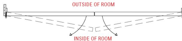
\*BOTH DOORS HELD IN CLOSED POSITION BY ROLLER CATCHES (INCLUDED) IN THE TOP OF THE DOORS. NO HANDLE/LOCK BORING.
