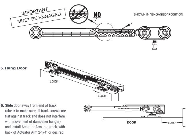
position from Jamb. **HAND TIGHTEN** (do not use power drill) Actuator Arm on track. Check to make sure Arm stayed straight in track. Slowly close door, checking to make sure door touches Jamb, if not. Slide door away from Jamb and readjust Actuator Arm. Slowly close door again, checking to make sure soft close is working properly. Once confirmed, begin using door normally.
